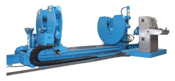
Forum Energy Technologies' AMC double-top open (DTO), high-torque stroking (bucking/makeup/breakout) machine is a self-contained, free-standing, hydraulically powered unit designed for fast and accurate makeup and breakout of threaded connections on drilling tools, well completion assemblies and other oilfield related equipment, up to a maximum torque of 100,000 ft-lb.
