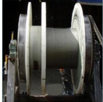
inner armor into the plastic core before the outer armor is applied. This process reduces the diameter changes typical of a new cable, which starts the seasoning process in advance of running in a well. See the picture to the right. The insulation, depicted in red, shows the indentation made during the manufacturing of Quality Cables.
