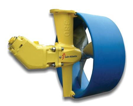
Forum's Sub-Atlantic™ range of hydraulic thrusters has become the preferred propulsion for ROV's and cable burial/ maintenance vehicles. Working in a highly aggressive environment, they have earned a reputation for reliability, efficiency and exceptional performance.
