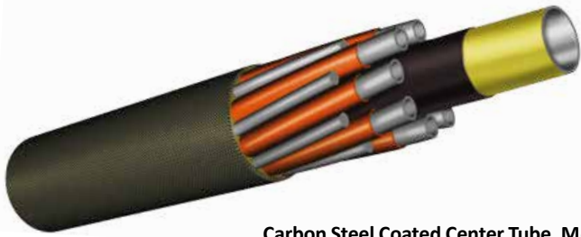
Carbon Steel Coated Center Tube, MeOH and LDHI Injection Lines and Umbilical Gaslift Tubing
