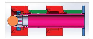
The ball is free to float upwards, significantly reducing the shockloading due to casing movement (sudden stops/starts) and allowing back flow circulation to clean out the Collet/sleeve bore by exposing full sleeve ID.
