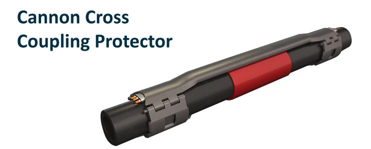
Cannon Cross Coupling Protectors protect and support many configurations of control lines, ESP cables, umbilical lines or encapsulated bundles. The Protector uses a channel to shield cables and lines as they transition across the coupling to prevent damage during installation and retrieval. The compressive fit design accommodates undersize and oversize tubing per API specification and secures the cable or lines to the tubing.
