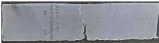
ID corrosion pitting and fatigue cracks
