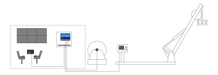
Scantrol AHC is installed as a replacement of one of the existing control stations, which means it is possible to have a very efficient installation process. There is no need to change any of the original control functionality.
