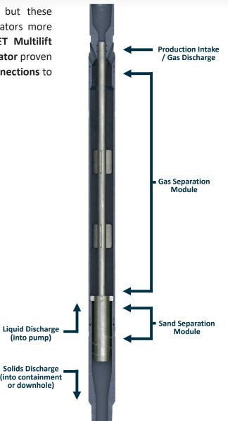
With the steady demand for enhanced oil production, artificial lift protection is critical for today's operations. Multi-tool systems are available, but these antiquated units pose long-term issues that ultimately cause operators more money and downtime. Designing an innovative solution, the **FET Multilift Solutions Pump Saver Plus delivers an all-in-one gas and sand separator** proven to **extend run life** and **eliminate the need for multiple tools and connections** to make up the BHA.
