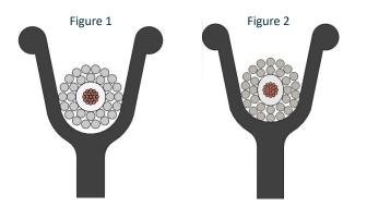
When applying tension in Figure 2, the wireline pulls down into the groove and deforms to the shape of the groove. This permanent deformation can result in an "out of round" wireline where several issues can occur, including:
