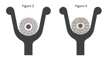
When applying tension in Figure 4, the wireline flattens into the groove and can permanently deform, causing:
