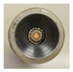
Viscous grease is injected into the assembly at pressures exceeding wellbore pressure and fills the space between the wireline and the inner diameter of the flow tubes. The grease packed in the tight annular space provides significant resistance to wellbore pressure by adhering to the surfaces of the cable and the flow tubes while
