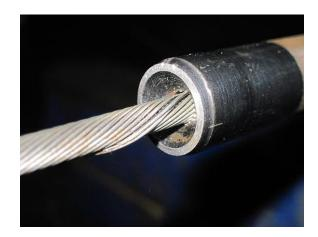
The crossed armor wire could also be forced back through the flow tubes by indenting the outer armor into the inner armor and plastic conductor, again going unnoticed. In this
