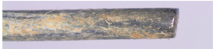
Broken armor wire from H_2S embrittlement
