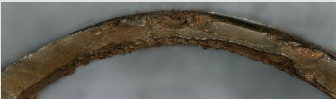
Metallography of field tubing showing dissolution of the longitudinal weld seam and heavy corrosion on the outside and inside surfaces.
