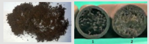
Metallography shows deep corrosion pitting in the base material 5-30% of nominal wall on both OD and ID.
