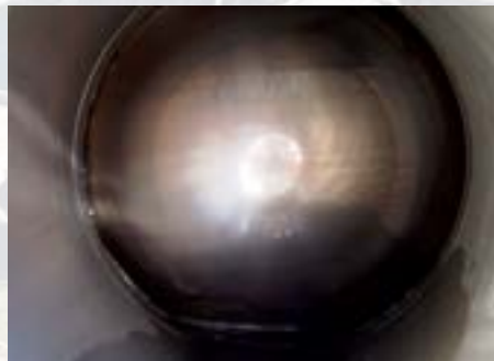
Close-up view of primary sealing surface of closed ball after approximately 1500 cycles at 2700 psig working pressure.
