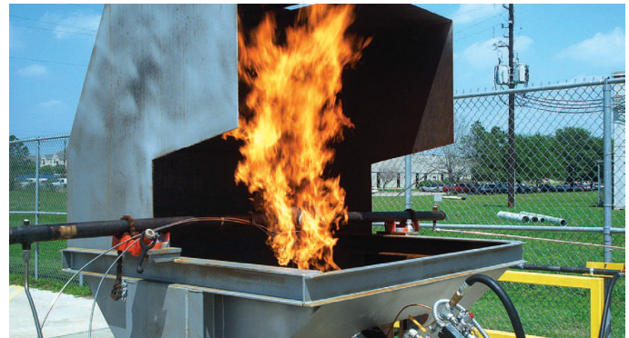
All Series 5312 valves meet API fire-safe standards.
