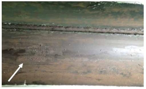
Note small colonies of corrosion with preferential pitting are reveal after pigging. Frequent removal of scale will reduce the amount of localized bacteria growth.
