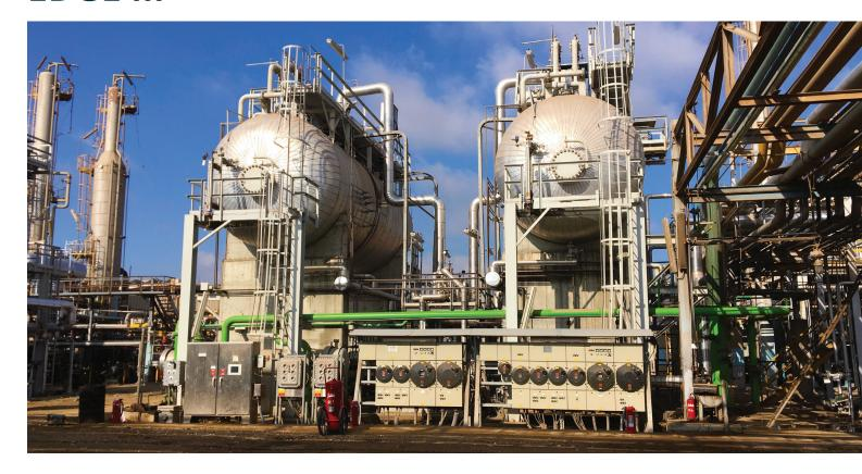
Processing different crude slates demands technologically advanced desalters that can accommodate a broad range of emulsion types. If the desalter is slow to react to varying feedstock properties, flow rates or water content fluctuations can spike operating costs.
