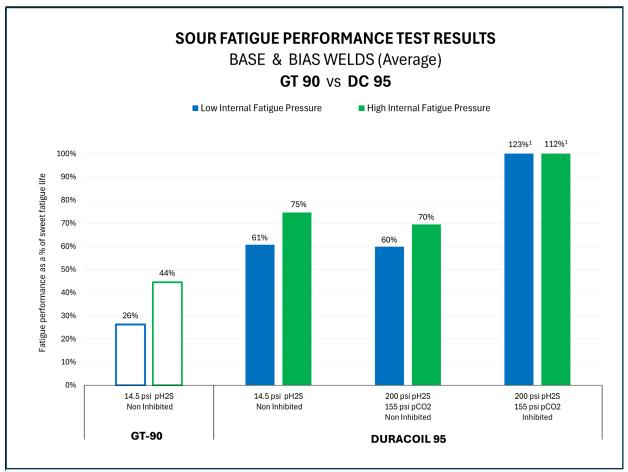
When GT-90 conventional Coiled Tubing is compared to DURACOIL 95 at ambient conditions, DURACOIL 95 shows better performance. Additionally, the remaining fatigue life of DURACOIL 95 after exposure to high partial pressures of H2S, with and without inhibitors, continues to demonstrate superior results in comparison to GT-90.
