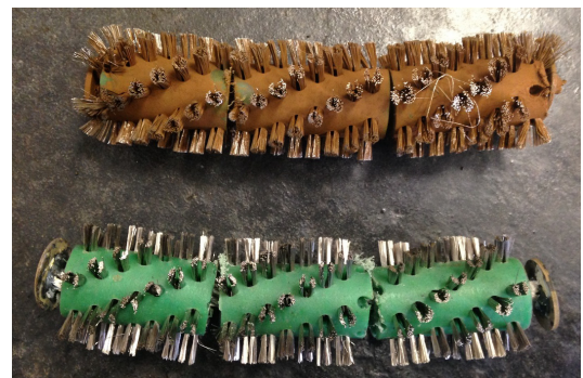
Brush pigs before (below) and after (above) pumping through CT.
